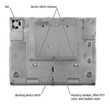
**FAN** — The computer uses an internal fan to create airflow through the vents, which prevents the computer from overheating.
