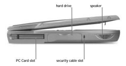
**PC CARD SLOT** — Has two connectors that support various types of PC Cards, including modems and network adapters. For more information, see the Tell Me How help file. To access the help file, see page 56.
